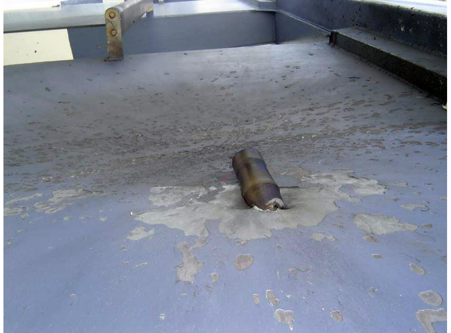
THE MOTOR OF A ROCKET-PROPELLED GRENADE (RPG), SHOWN AFTER STRIKING THE SEABOURN SPIRIT
